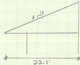
$\Rightarrow$  Load per unit length is to be distributed over a distance of 15 ft from the upper roof eave
