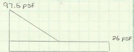
Snow drift on interior walls of fake Mansard Roof
