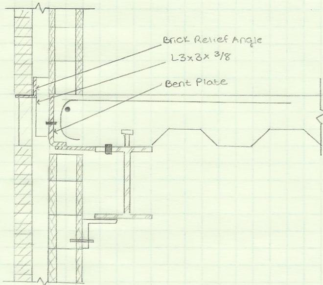
The exterior brick load is taken by the relief angle and transferred into the L3x3x 3/8. From there the load goes into the bent plate at the slab edge and into wide flange beam. The CMU load is also transferred into the beam through the bent plate. From there the load is transferred into columns and down into the foundation.
