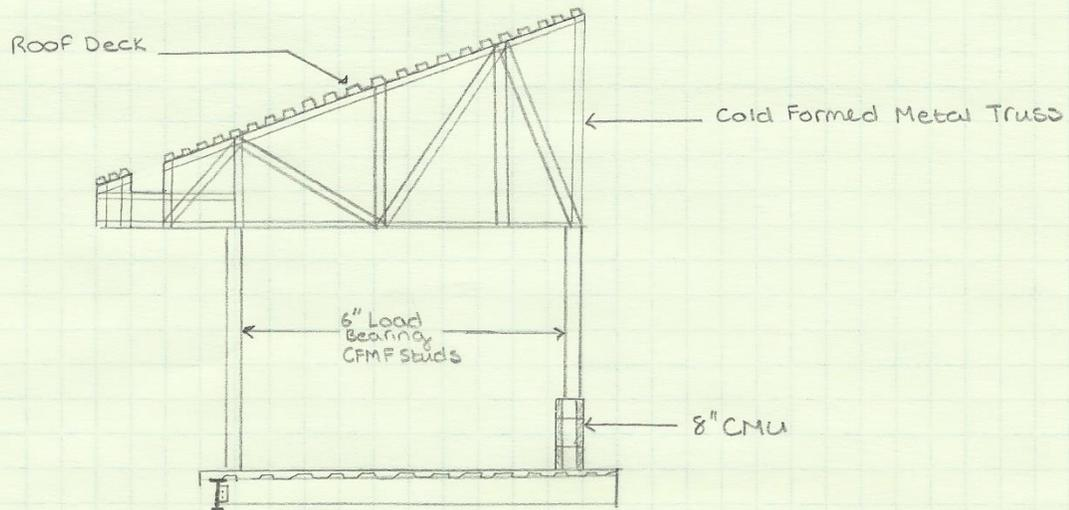
Distributed line load from CMU wall bearing trusses
